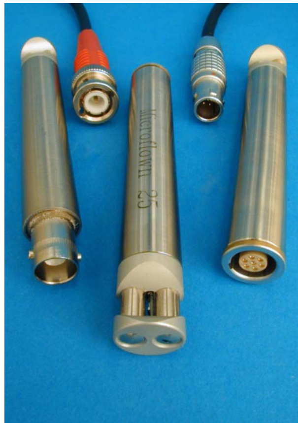
Figure 1-6: Different types of 0.5-inch packaged microflowns. At the left, an ICP® powered microflown is visible, in the middle and right, microflowns with LEMO® connectors are shown.
