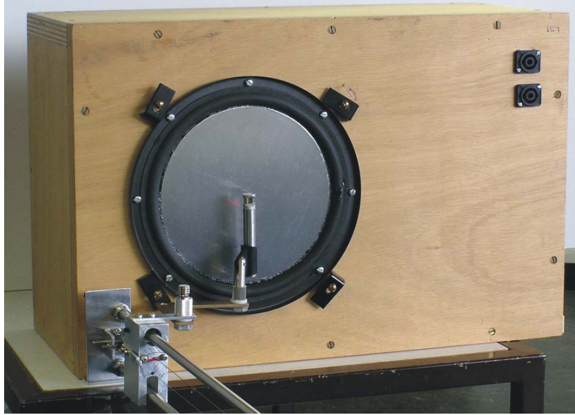
Figure 5-37: Measurement setup: a loudspeaker with an aluminium plate glued on and the p-u probe on a traverse robot.
