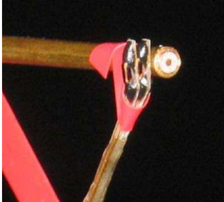
Figure 5-9: Pressure microphone (Microtronics 8001) and the two particle velocities sensors used. The three sensors are positioned as close as possible to each other.
