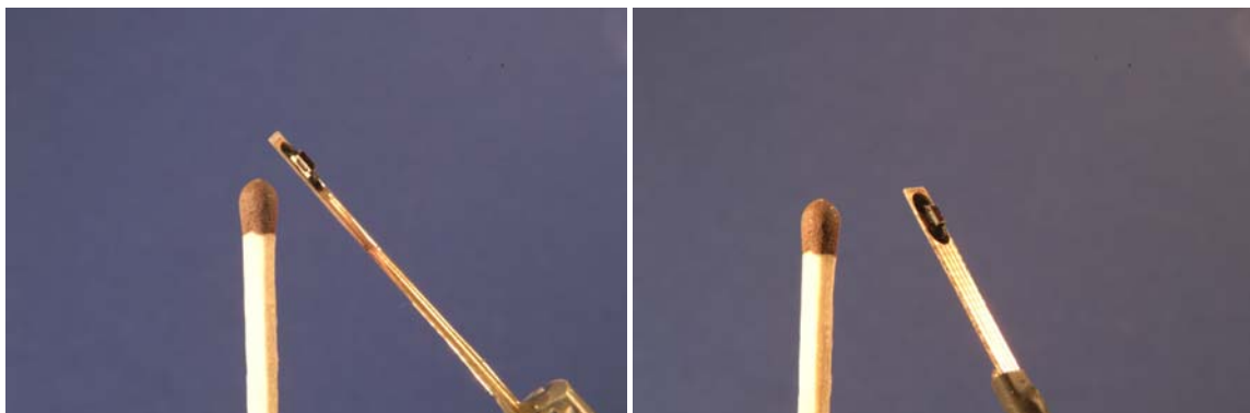
Figure 1-9: Photograph of a scanning probe (courtesy Microflown Technologies BV.). Left: old two-wire sensor, Right, the new microflown sensor.
