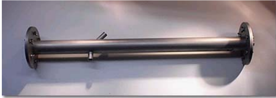
Figure 2-1: Standing Wave Tube available for three-dimensional calibration of multi-microflow sensors (source: Microflow Technologies). Notice the extra 0.5 inch opening needed for the three-dimensional calibration technique (see section 2.3.5) or microflows placed under 45 degrees.
